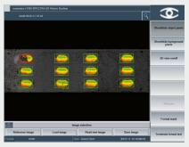
Evaluation of pockets filled to the rim. Missing powder is detected by the system.
