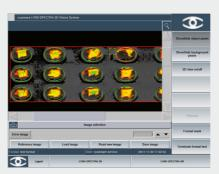
Evaluation of a blister filled with powder pellets. Any pocket with insufficient fill of powder is detected despite the irregular shapes the powder takes in the pocket.
