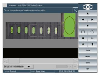
Camera-specific colour tolerances can have a negative impact on evaluation. The software feature "Colours per Camera" determines that colour values are set for each camera individually during teach-in. This eliminates camera-based irregularities and facilitates precise evaluation. The user, however, teaches on one image.
