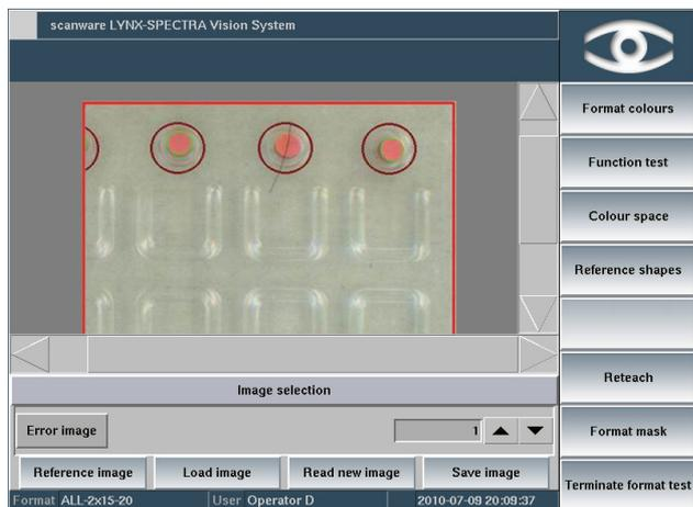
Presence of hair is detected as a wrong colour and causes ejection. The recognition power depends on inspection area and image resolution.
