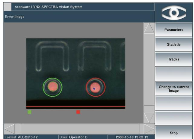
Products with minimal defects, such as a polishing error or surface defect, are detected by **SPECTRA Japan Quality**.
