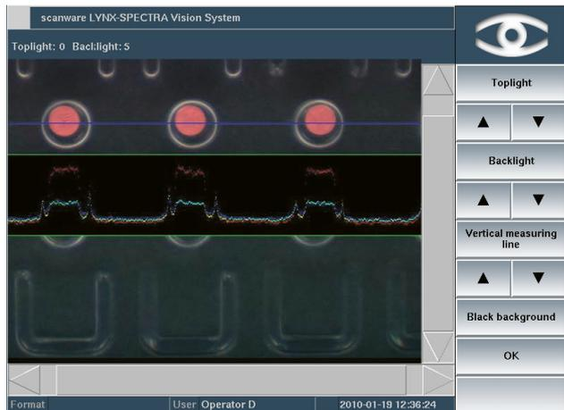
For Japan Quality Product Inspection, even the slightest degree of reflections can be problematic. The measuring line used by scanware enables the setting of safe, reproducible settings for the W-LED illumination. The line can be used vertically, for example if multiple camera images appear one underneath the other.
