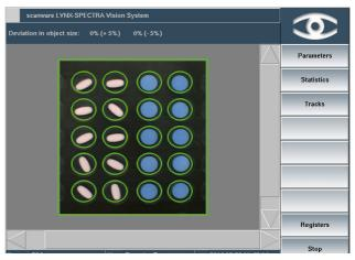
Products with various shapes in the same blister can be inspected simultaneously. To do so, product-specific parameters are set.
