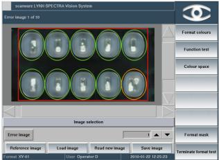
The use of x/y measurement is important for various products, for example Medical Strips. For hard gel capsules with heterogeneous filling, varieties in distribution of products within the capsules can be evaluated.
