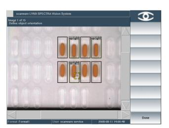
The recognition of upright objects reduces product ejections. Upright objects are identified as correct rather than ejected as too small.
