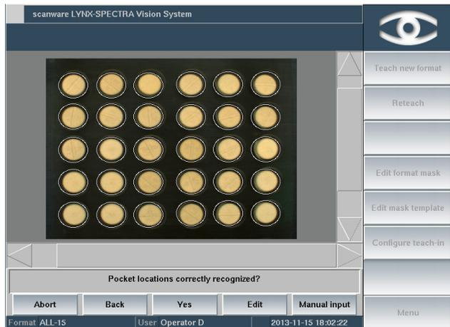
Automation of the teach-in simplifies the process so production can start in minimum time. Object position, blister geometry and product color are recognized automatically. A manual teach-in is also possible.
