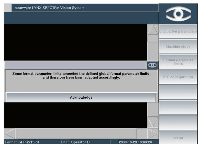
Tolerances can be set on a global level by the administrator. Thus, the user can only operate within these global parameter limits when making changes. This increases production security.
