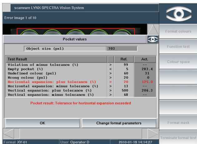
During format testing, pocket-specific values of deviations are displayed. This allows a precise analysis of faulty products.
