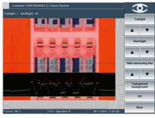
For the inspection of labels, a designated illumination setting can be chosen independent of the ring code inspection.
