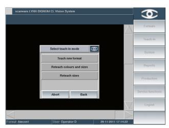
The guided teach-in is particularly easy to follow. The inspection areas for individual criterions can be defined individually. Using test runs and format testing, the evaluation can be checked.
