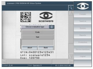
Teach-in can be performed very quickly. Firstly, the print type to be inspected is chosen. Thereafter, only the parameters relevant to the type of print need to be taught.
