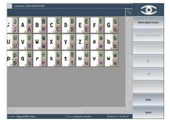
The unicode library does not grow continuously which would slow down evaluation. Instead, evaluation is based on an intersection of parameters of the previously read variants. Thus, the evaluation speed is uniformly fast.
