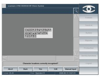
In OCV mode, the system automatically recognises the position of the text.
