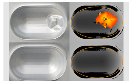
Photo and evaluation view of blister inspection
