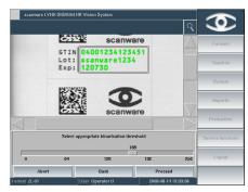
The OCR camera system is fully formatindependent. scanware has chosen a featurebased recognition process. The object to be inspected is analysed based on features such as size and centre of gravity.
