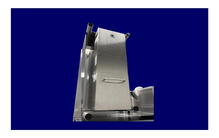
The Print Inspection SIGNUM HR is a highly efficient greyscale vision system and the complete solution for on-line 100% optical inspection of print including characters (OCR) on packaging materials. It offers recognition capacity, operating features and operator comfort that exceeds that of most other vision systems. The high reading speed, integrated illumination and outstanding software make the system the best of its kind.
