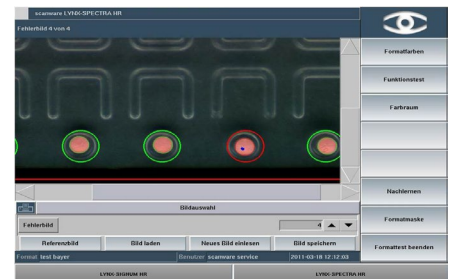
Example of detection of a surface defect
