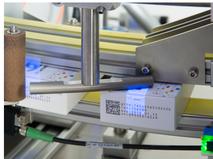
High precision of label placement thanks to precise folding box guidance
