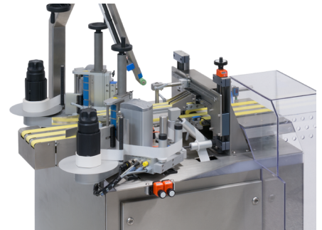
Tool-free adjustment to folding box size
