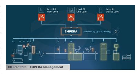
Further IMPERA Line Management undertakes all data transfers between the manufacturer's data base and the devices. In detail it imports data from the producer's data base, processes it and re-transfers it after completion. This makes the system ideal to fulfill serialization requirements which are mandatory for European pharma companies as well as contract packagers as defined in the Pharma Directive EU/2011/62 ("Falsified Medicines Directive").
