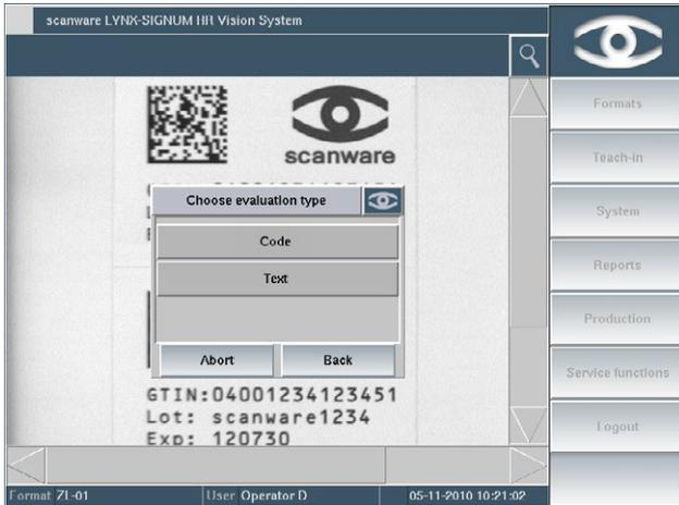
The teach-in can be configured and consequently is very fast. Firstly, the print type to be inspected is chosen. Thereafter, only the parameters relevant to the type of print need to be taught.
