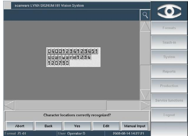
In OCV mode, the system automatically recognises the position of the text.
