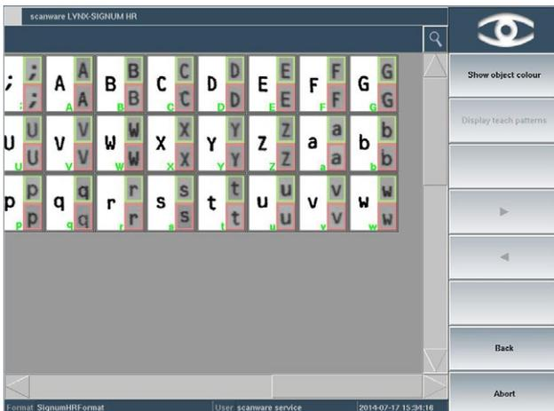
The unicode library does not grow continuously which would slow down evaluation. Instead, evaluation is based on an intersection of parameters of the previously read variants. Thus, the evaluation speed is uniformly fast.
