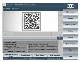
The evaluation of faulty codes clearly states the deviation so the problem can be resolved and ejects minimised.
